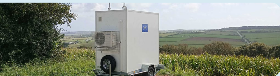
Example of a mobile station for measuring ammonia and PM10 fine particles, installed on the South site.
